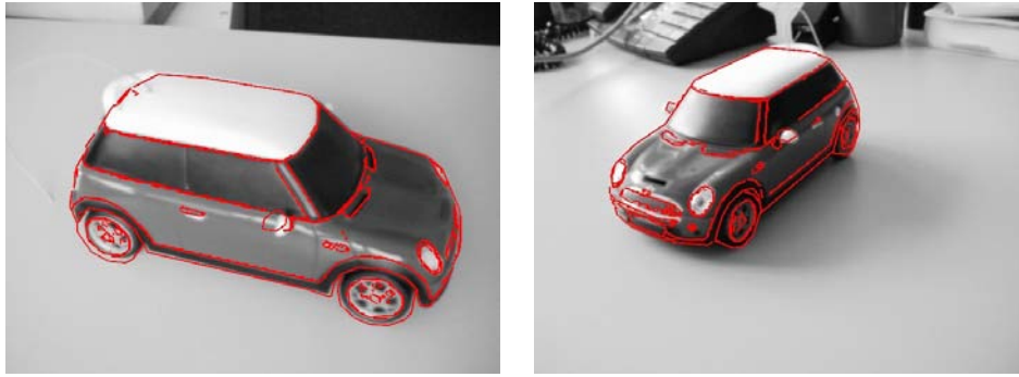
Figure 5.9.: Tracking a toy car by using the frame-buffer approach.
