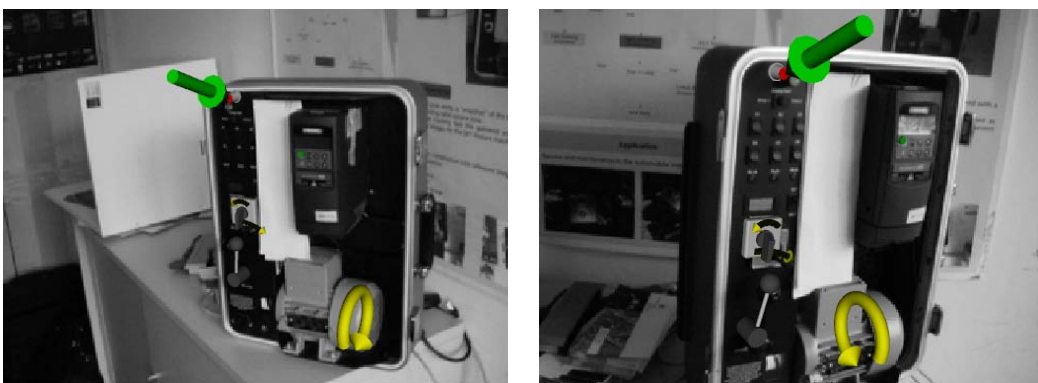
Figure 6.11.: A virtual augmentation is rendered with the estimated camera pose onto the camera image. If enough KLT-features can be tracked, the virtual arrows are always overlaid correctly in the scene.
