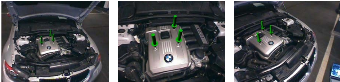
Figure 6.14.: Tracking of a motor engine. The arrows are rendered with the camera pose, which is obtained from the KLT-feature tracking.
