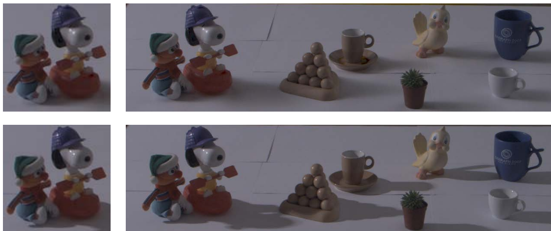
Figure 7.6: Arbitrary reference object (left, 128 \times 128 pixels), sparse sampling: an arbitrary part of the scene can be used as a probe object in the case of a fixed camera setup. The top row shows the reconstruction for sparse sampling ( n = 250 ), the bottom row ground truth. While the sparseness causes blurred highlights and shadows, the reconstruction does not produce multiple blended shadow boundaries or comparable artefacts as point-based lighting sometimes does.
