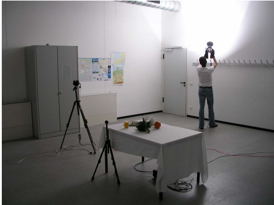
Figure 7.4: Measurement setup for the still camera: an Olympus C5050Z digital camera records objects on a table which are indirectly lit by a hand-held spotlight pointed at the white walls, ceiling and floor. The reference object, a black snooker ball, is mounted on the small tripod next to the table.
