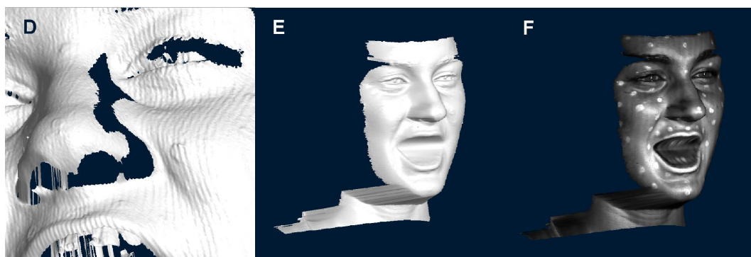
Fig. 6.3. Data preprocessing Detail of the mesh obtained from the scanner with holes and residues of the projected line pattern (D), reconstruction with tongue and teeth information removed, holes filled and geometry smoothed (E), reconstruction with average texture (F).
