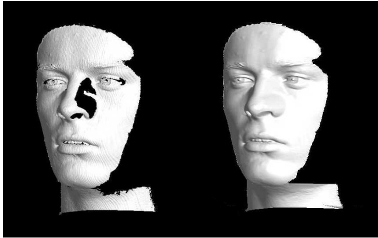
Fig. 7.5. Hole filling and scanning residues smoothing This figure illustrates how the holes in the original recorded data (left) can be filled and adapted to the surrounding topology (right). This adaptation is obtained by smoothing the filling with a binomial kernel. The same procedure is performed on the full geometry in order to remove the residual noise from the acquisition. The smoothing is able to keep the details of the eyebrows and of the eyelids.
