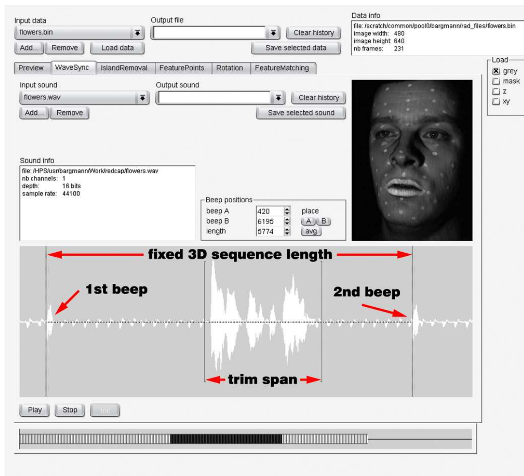
Fig. 8.9. Our interface for sound synchronization The original 3D sequence is aligned according to the the beep tones which insures an exact matching with the audio track. The user then selects the subsequence of frames to be retained (bottom panel): the waveform shows the position of the speech information, the visualization window is updated as the user moves the cursors so that these can be accurately placed before the start and after the end of the articulation movements. The lower panel highlights in black the frames which are retained.
