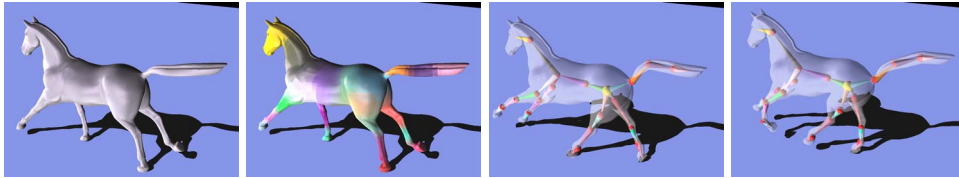
Figure 14.1: From left to right: Input animation, color-coded distribution of blending weights, and two poses of the input re-generated based on our skeleton-based version.
