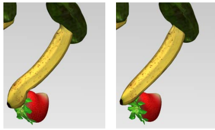
Figure 15.4: With larger offset segments, the fruits in the horse’s leg deform more stiffly (right) than with tighter offsets (left).
