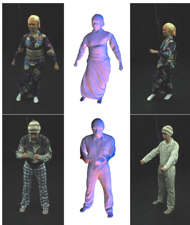
Figure 9.6: Side-by-side comparisons between an input video frame and the pose of the laser scan that our approach reconstructed. The poses of the persons and even the deformations of complex apparel, like the kimono, are faithfully reproduced.
