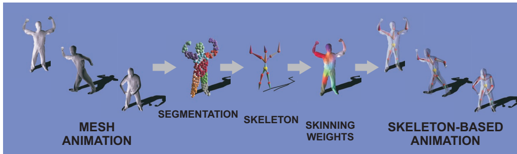
Figure 14.2: Overview of our algorithm: using an animated mesh as input, our approach segments the model into plausible approximately rigid surface patches (shown in different colors), estimates the kinematic skeleton (joints shown in red) and its motion parameters, and calculates the skinning weights connecting the skeleton to the mesh. The output is a skeleton-based version of the input mesh animation.
