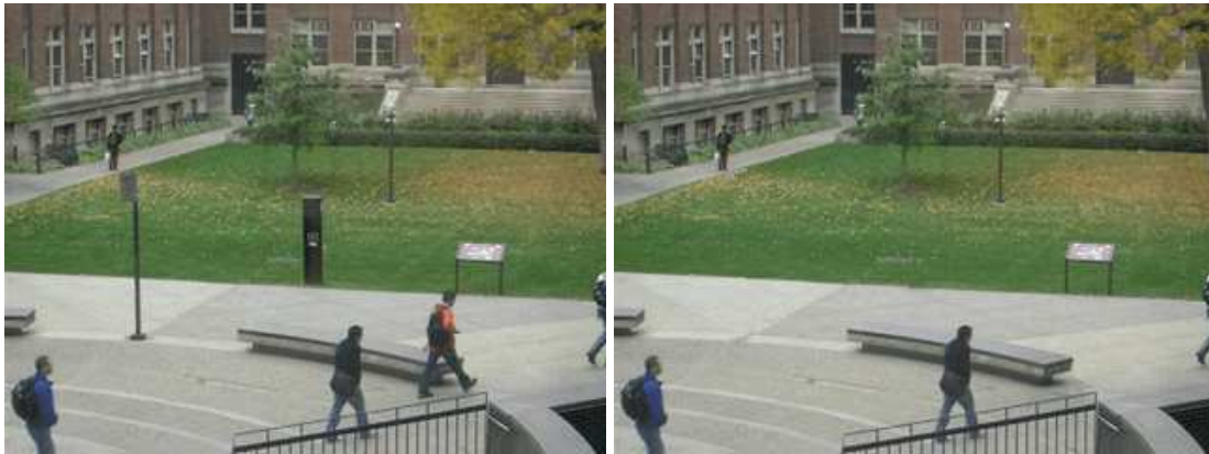
Figure 2.6: Left: Original video frame from [PSB05]. Right: inpainting result (person was removed). © K. Patwardhan, G. Sapiro, M. Bertalmio, used with permission.
