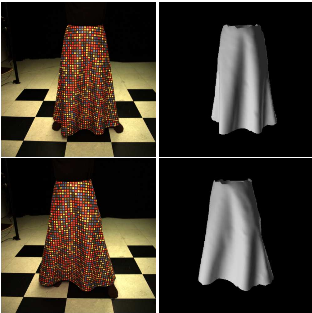
Figure 4.15: The reconstructed surface faithfully represents the cloth folds visible in the input frames.
