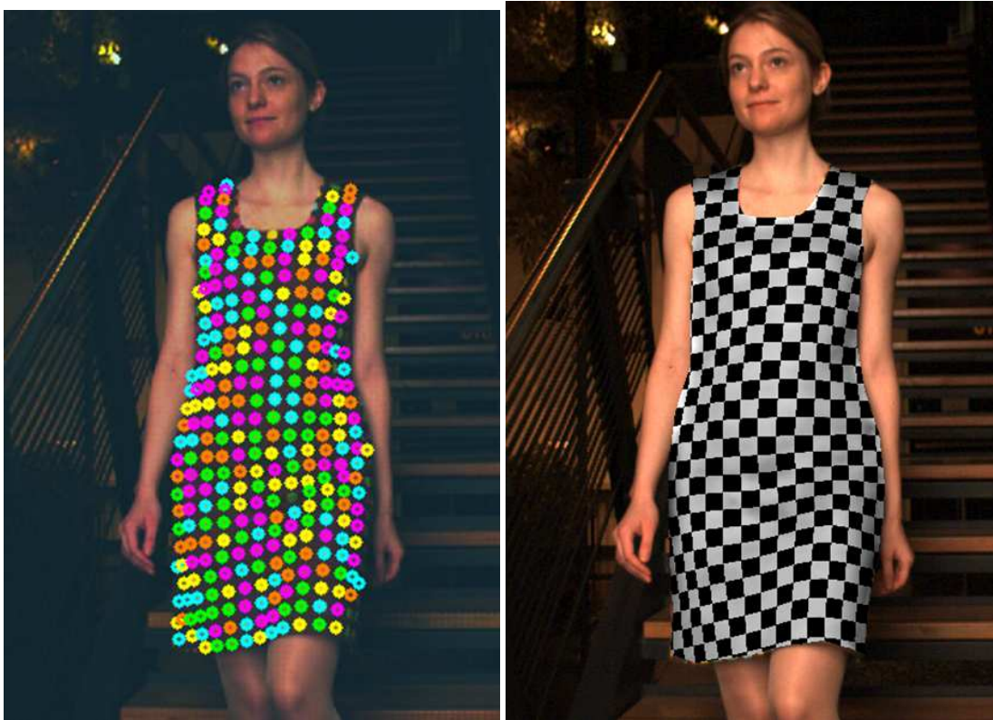
Figure 5.5: Texture Coordinate Interpolation: The feature positions (left) are interpolated to obtain a uv parameterization of the garment (right).
