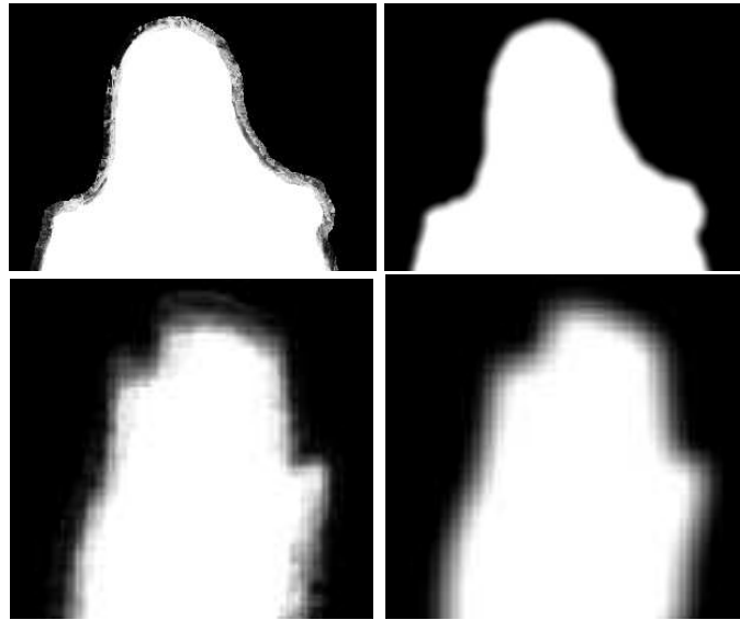
Figure 6.11: Results from our border matting algorithm. Left column: raw alpha mattes. Right column: regularized alpha mattes.
