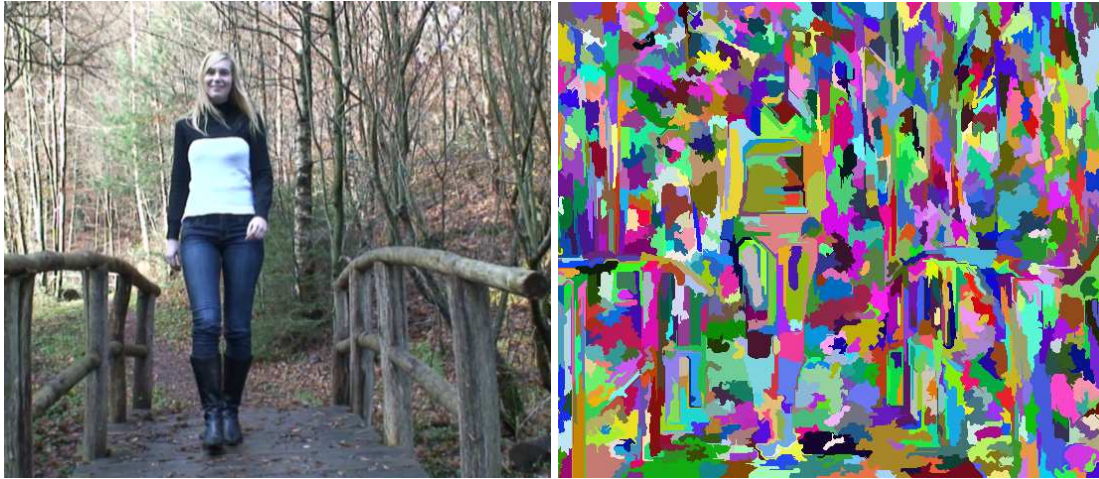
Figure 6.3: Result of segmentation during preprocessing. Left: input image, right: segmentation result, each colored region is a superpixel.
