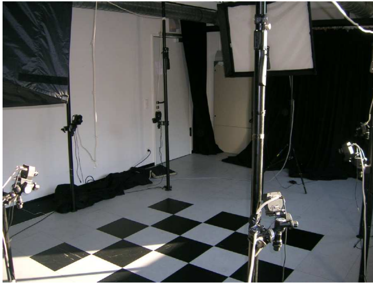
Figure 4.9: Camera setup using eight cameras and two HMI lamps with softboxes.
