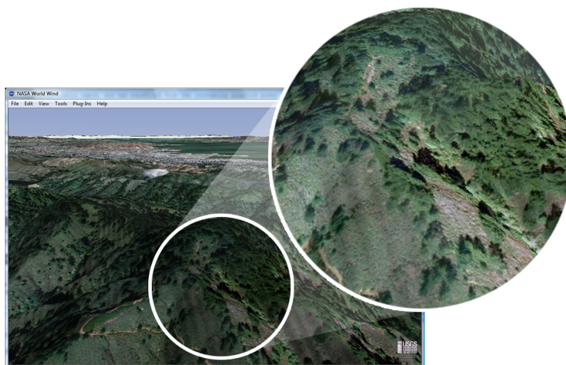
Figure 1.1: Orthophotographic maps projected onto a terrain model become apparently 'flat' when viewed at low angles.
