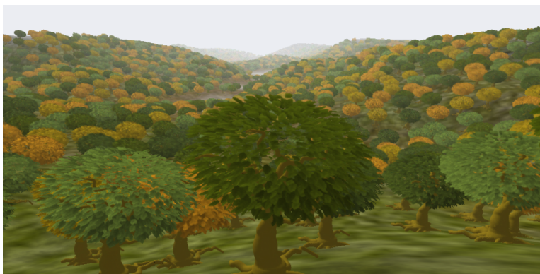
Figure 2.9: Sample scene rendered using Deferred Splatting [GBP04]. The scene contains approximately 2300 visible trees consisting of approximately 750k polygons each. It is rendered at 11fps.
