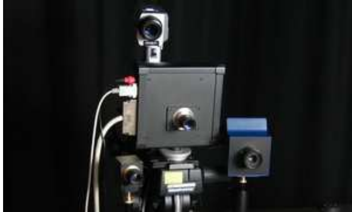
Figure A.1: Cameras used in our experiment: HDRC VGAx (lower left), Silicon Vision Lars III (center), Jenoptik C14 (lower right), and Minolta LS-100 luminance meter (top).
