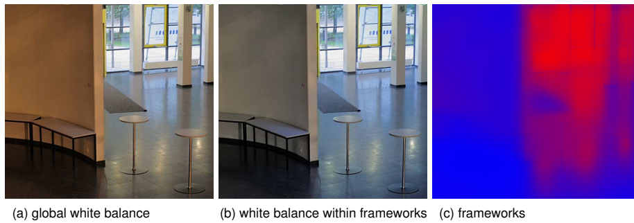
Figure 5.10: The daylight from a cloudy sky dominates the white balance in image (a) and causes the orange color cast in the interior illuminated by a tungsten light. The frameworks (c) can be used to separate such areas of different illumination and to perform an independent white balance in each of them (b).
