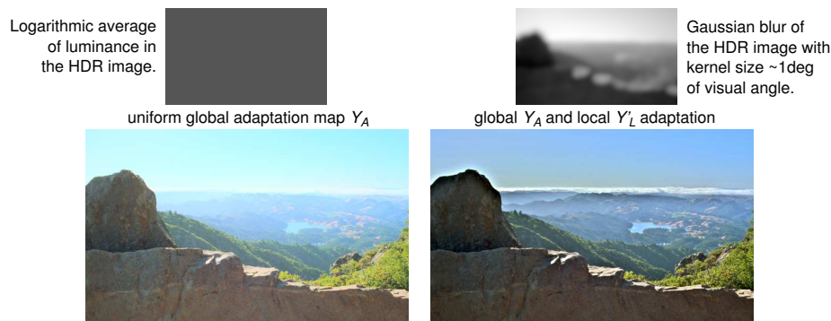
Figure 2.5: Tone mapping result with global, equation (2.1), and local adaptation, equation (2.3). The local adaptation (right) improves the reproduction of details in dark and bright image areas, but introduces halo artifacts along high contrast edges.
