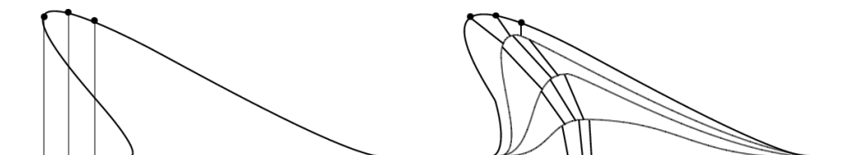
Figure 4.9: If the high-frequency detail cannot be projected onto the successive level (top), intermediate levels have to be inserted to guarantee a feasible detail reconstruction (bottom).
