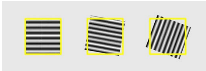
Figure 3.16: The rotating operator over the sample, generates diamond structures, whose border windows need to be cut away.
