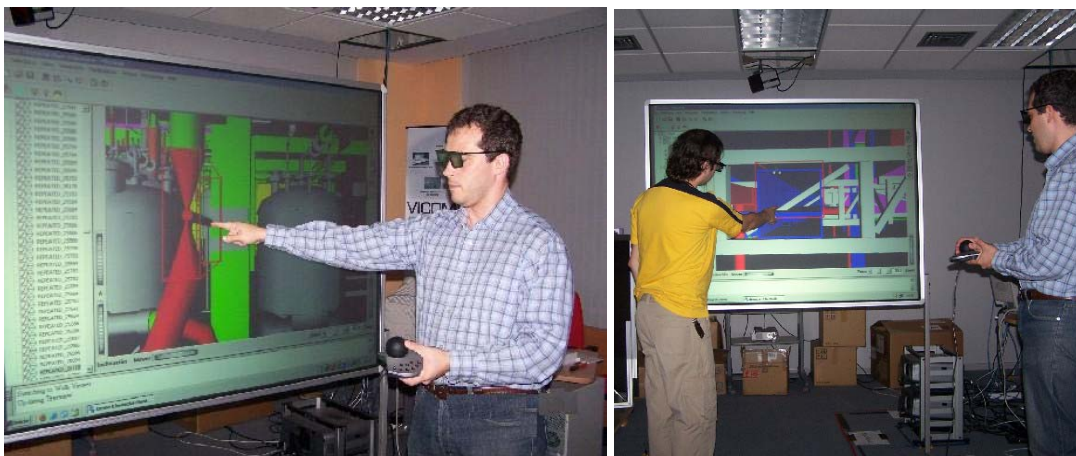
Figure 89. The Mirowalk system in a simple VR setup with passive stereo and back-screen projection, using a SpaceMouse as input device.
