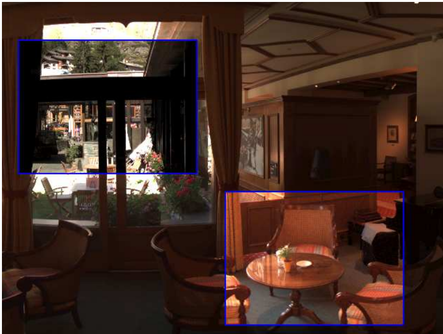
Figure 5.15: CAFETERIA sequence, dynamic range -1.9 \div 3.6 [\log cd/m^2] . The background frame is clamped to a displayable range. Our dynamic range exploration tool, visible as two windows, shows a luminance range -1.0 \div 1.0 [\log cd/m^2] (lower right) and a high luminance range 1.0 \div 3.0 [\log cd/m^2] (upper left). Details in these windows are not visible in LDR video. The source panorama courtesy of Spheron, Inc.
