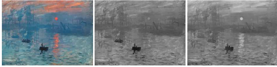
Figure 6.14: An example of a saliency preserving color to gray mapping. Left – original image; center – luminance image; right – the result of the color to gray algorithm. Image: Impressionist Sunrise by Claude Monet
