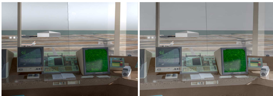
Figure 6.17: The algorithm by Fattal et al. [2002] (left) renders windows panes of different brightness due to the local nature of the optimization procedure. The contrast compression on the multi-scale contrast pyramid used in our method can maintain proper global contrast proportions (right). Image courtesy of Greg Ward.
