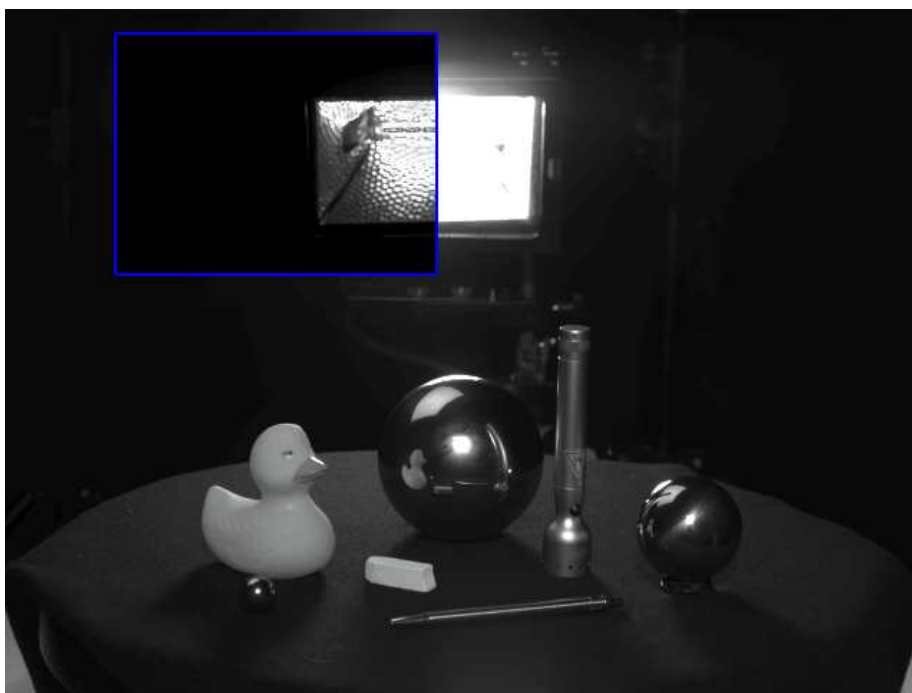
Figure 5.16: LIGHT sequence captured with the HDR video camera, dynamic range 0.3 \div 4.9 [\log cd/m^2] . Details of the halogen bulb are well preserved despite high luminances. The visible range in exploration tool window is 2.9 \div 4.9 [\log cd/m^2] .
