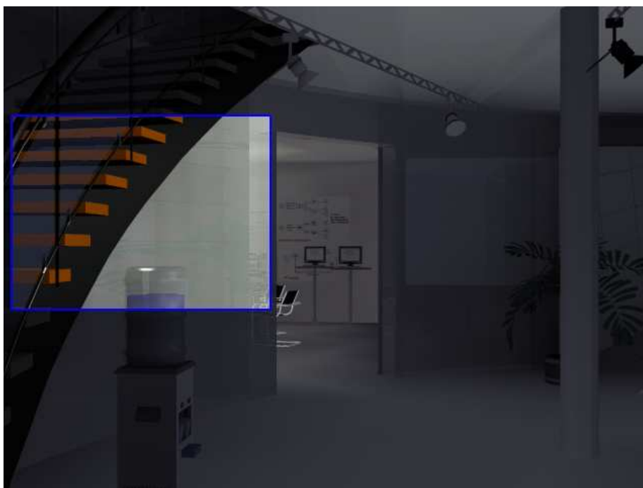
Figure 5.14: OFFICE sequence with simulated low-level lightning, dynamic range -4.0 \div 0.2[\log cd/m^2] . The main frame is tone mapped using the Pattanaik et al. [Pattanaik et al. 2000] algorithm. Lack of colors and the bluish cast are due to the night vision post-processing as proposed by Thompson et al. [Thomspon et al. 2002]. The exploration window reveals color and details in the -2.2 \div -1.2[\log cd/m^2] range. The scene model courtesy of VRA, GmbH.
