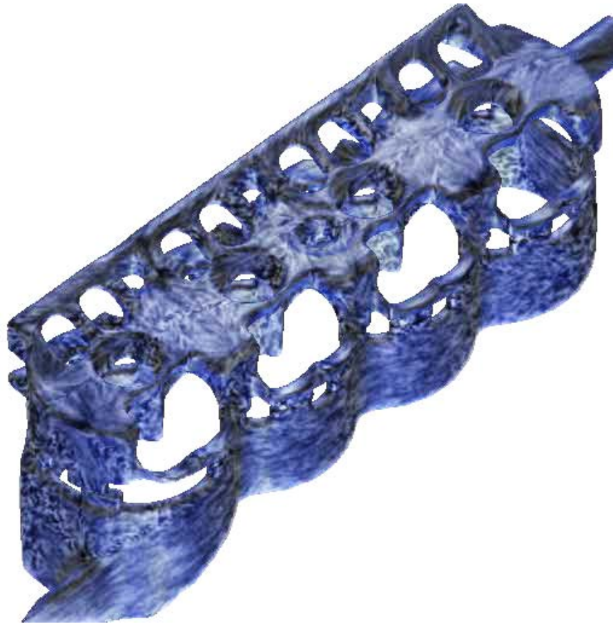
Figure 4.2: Visualization of flow at the complex surface of a cooling jacket -a composite of over 250,000 polygons.
