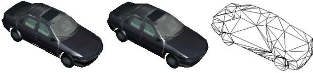
Figure 4.10: Left: original car model. Middle: the TDM representation. Right: the mesh of the TDM.
