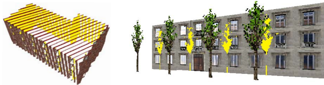
Figure 3.13: Examples for visibility culling within impostors. Culled texels are drawn in yellow. Left: house example. Note that even small occlusions visible in the windows and door frames are identified. Right: facade partly occluded by trees.
