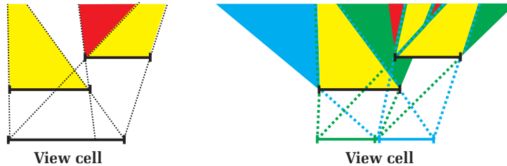
Figure 3.14: Left: example for occlusions caused by umbrae (yellow areas) and overlapping penumbrae (red area). Right: approximate occlusion (yellow areas) using the intersection of several umbrae obtained from a view-cell decomposition.
