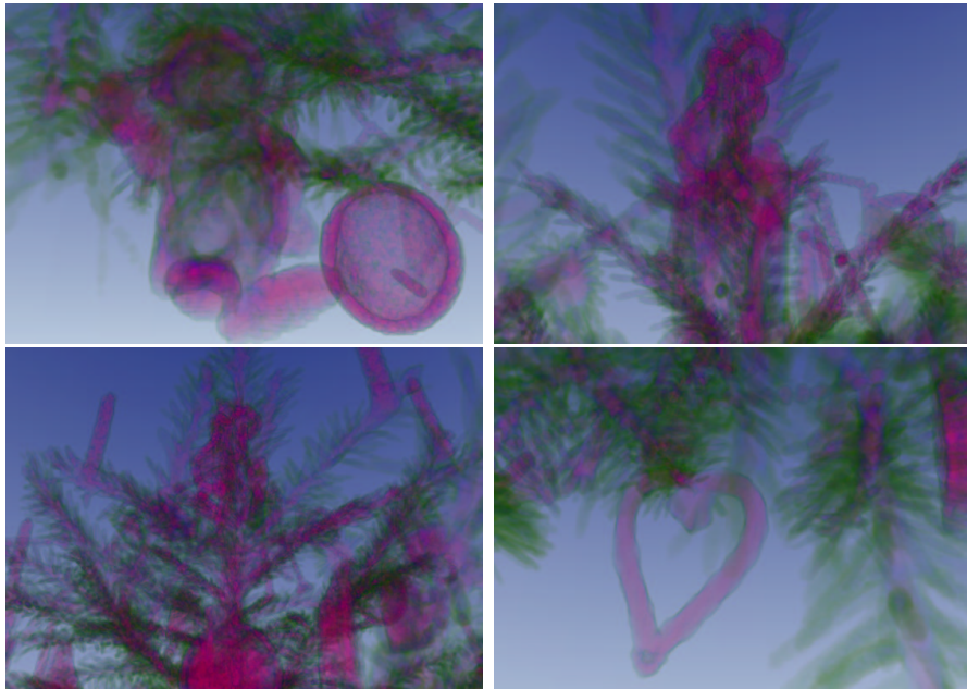
Figure 5.7: Viewdependent simplification with error threshold of 1 pixel. The tetrahedral mesh is rendered with pre-integrated cell projection.
