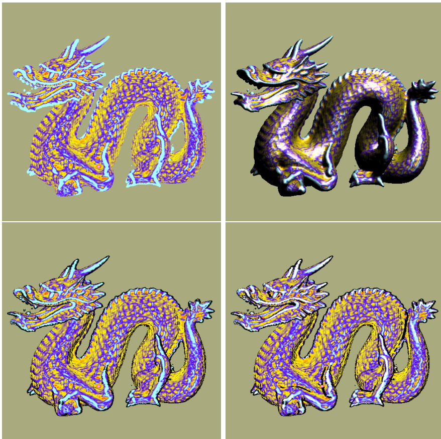
Figure 5.16: Dragon distance field (128x128x128) with colors from curvature magnitude (top, left); with Phong shading (top, right); with contours (bottom, left); with ridge and valley lines (bottom, right).
