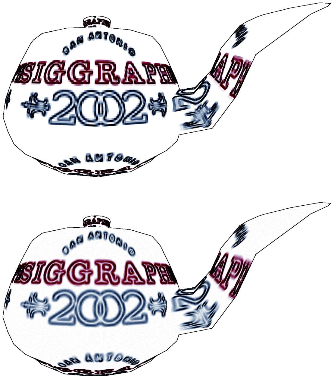
Figure 3.14: Teapot mapped with a 128x64 texture. (top) bi-linear interpolation; (bottom) high-quality reconstruction via 2D convolution with a bi-cubic B-spline; additionally, real-time convolution with a Sobel filter was performed in screen space to enhance edges.
