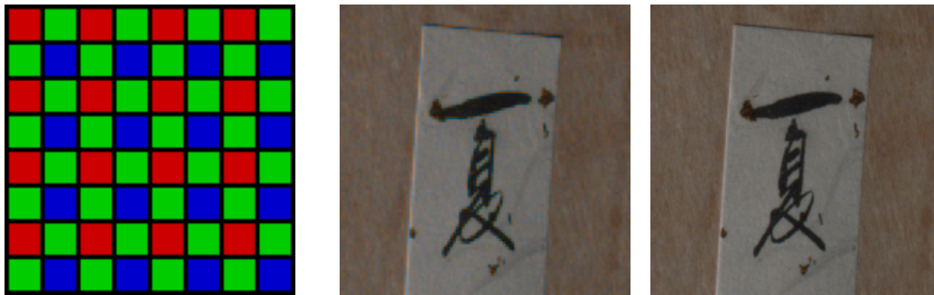
Figure 3.3: The Bayer pattern [Bayer76] for color image capture. Left: Arrangement of the individual color sensors. Middle: Color interpolation artifacts in an image acquired with a Bayer pattern sensor (Jenoptik ProgRes C14, single shot, fast reconstruction). Right: Ground truth image acquired using 4-shot mode. Note also the visually higher resolution of the ground truth image.
