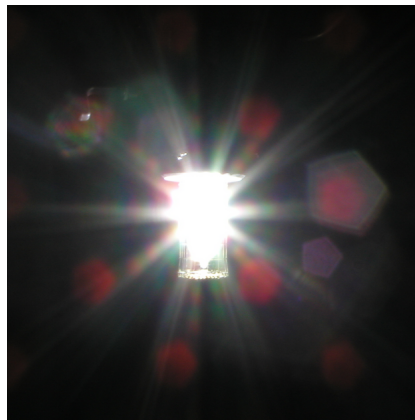
Figure 2.2: 10-sided star around a bright light source caused by diffraction at the edges of the camera lens' pentagonal aperture. The image also shows other effects such as lens flare caused by reflections inside the optical system.
