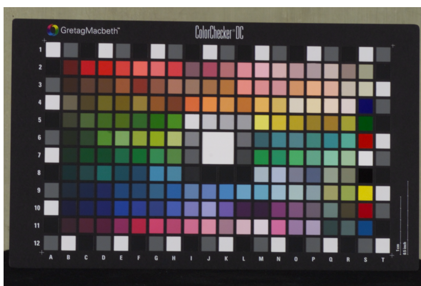
Figure 3.7: The GretagMacbeth Colorchecker DC used for ICC profile generation imaged under diffuse illumination.
