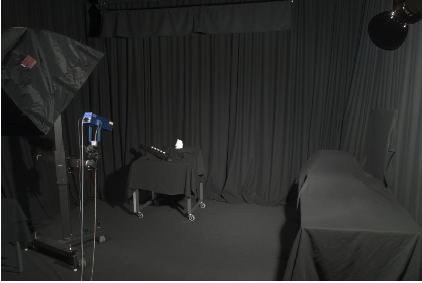
Figure 3.11: The acquisition lab at the Max-Planck-Institut für Informatik. A test object on the table is illuminated by two HMI light sources with different reflectors.
