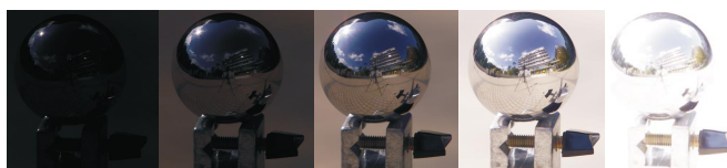
Figure 3.8: Sequence of images taken at various exposure times in order to reconstruct a single high dynamic range panoramic image. Pictures courtesy of Michael Gösele and Philippe Bekaert, Max-Planck-Institut für Informatik.
