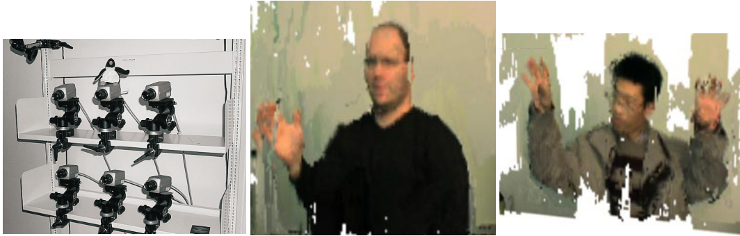
Figure 8.7: Left: Our Lumi-Shelf, consisting of a bookshelf, six consumer-quality Firewire video cameras connected to three Linux PCs, and one additional PC for rendering. Right: Some shots from an interactive Lumi-Shelf session, where the scene in front of the shelf can be rendered at near-interactive rates.
