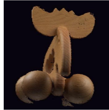
Figure 8.5: Synthetic view of a real-world wooden elk reconstructed using a voxel coloring technique. The images consist of 760 \times 502 pixels, and the display runs at 1 fps.
