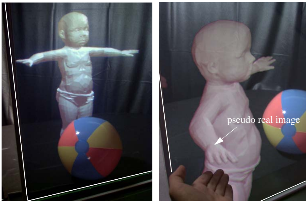
Figure 5.14: Left: Real objects behind the mirror (the ball) are illuminated and augmented with virtual objects (the baby). The angle between mirror and projection plane is 60^\circ . Right: Without attaching a clipping plane to the mirror, the baby can reach its arm through the mirror. The angle between mirror and projection plane is 80^\circ .
