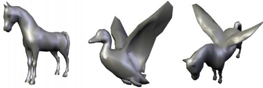
Figure 4.9: Using spatial control for modeling. A Pegasus is modeled by morphing between models comprising its features. Local morph control is used to define a transition state so that only the wings of the duck appear on the horse.
