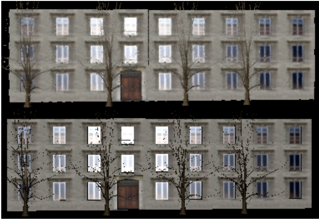
Figure 5.13: Note the correct filtering of the trees against the building front and the specular highlight in the windows for the impostor (top), and severe aliasing in the trees for geometry (bottom).
