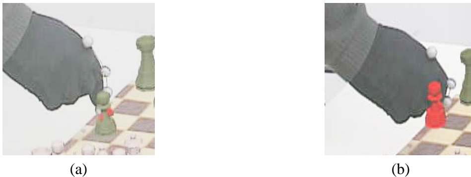
Figure 6.16: Manipulation of virtual objects by grab and release gestures: Natural interaction is possible using the finger tracker described in this section together with augmented reality displays. In this image, a user plays chess against the computer by moving virtual chess men with his finger on a real board.
