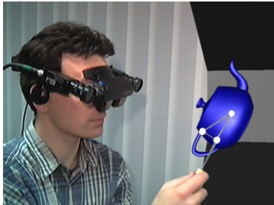
Figure 6.14: See-through HMD for inside-out tracking
