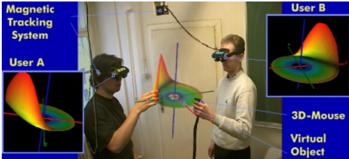
Figure 4: Two collaborators wearing see-through displays are examining a virtual object. Note that the system supports independent views on shared objects.
