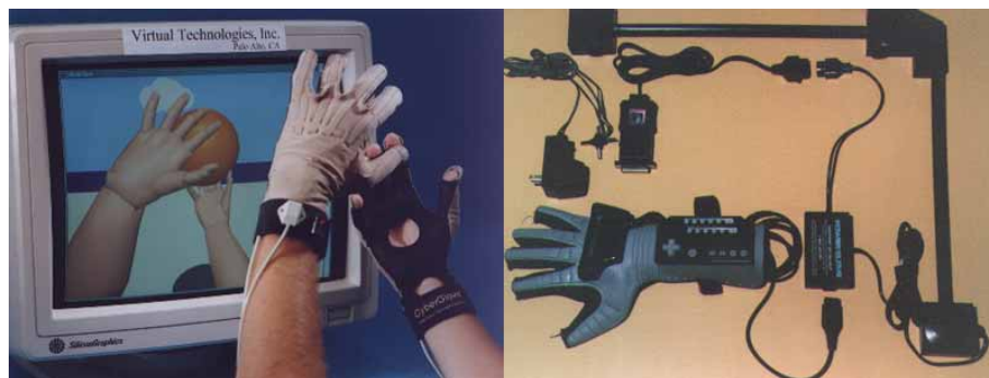
Figure 15. VTI CyberGlove and Mattel/Nintendo Powerglove .
