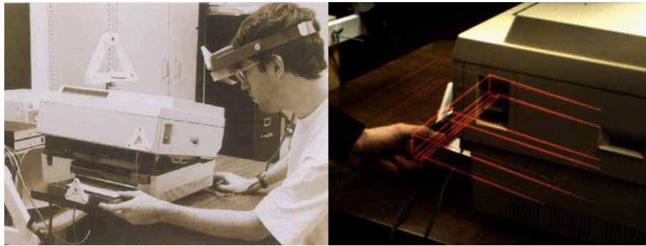
Figure 16. KARMA - the knowledge based AR-system provides situated visual help information.
