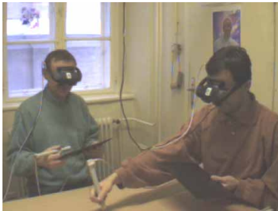
Figure 74. The hardware environment as seen from a non-participating observer. Each player wears a see-through head-mounted display and interacts with a Personal Interaction Panel.
