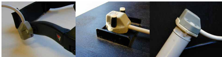
Figure 46. HMD and props equipped with a Polhemus Fastrak electromagnetic receiver.
