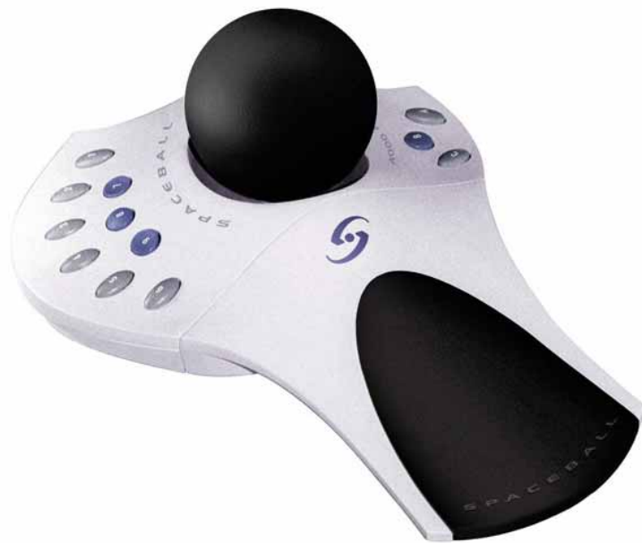
Figure 14. Spaceball 4000 FLX 6 degree of freedom input device.
