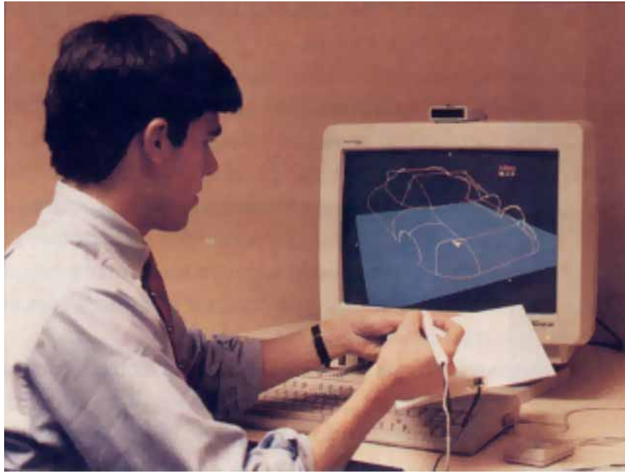
Figure 21. Designer sketching automobile parts with the 3-Draw interface, an early example of two-handed 3D-interaction device for desktop applications.
