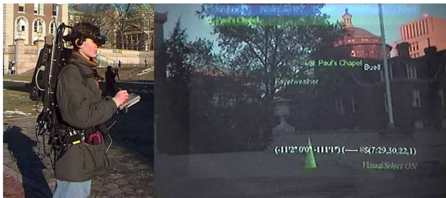
Figure 18. MARS – The Touring Machine allows browsing situated information in outside scenarios, e.g. the Columbia University.
