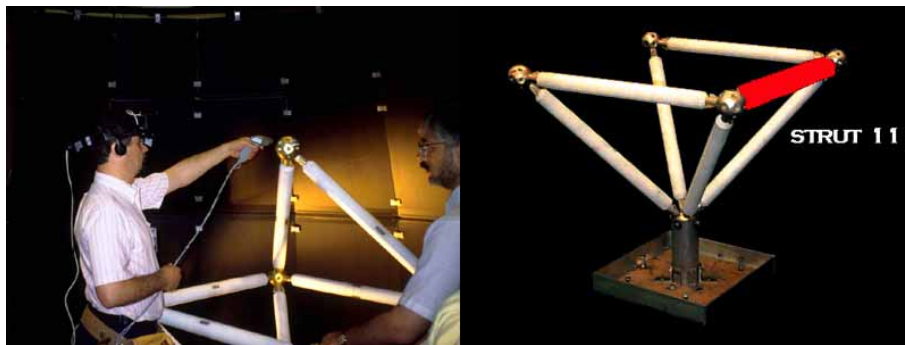
Figure 17. ARC – Constructing aluminum frame systems using augmented help information. A magnetically tracked bar-code reader provides interaction with the system.
