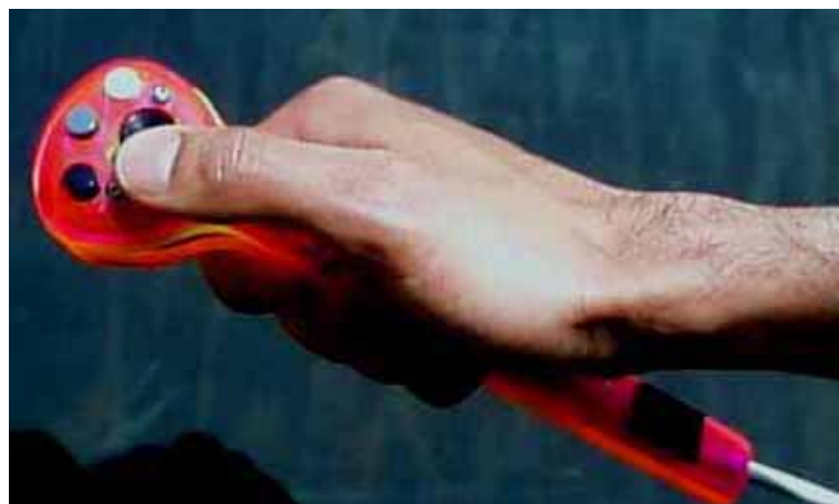
Figure 4. The wand used in most CAVE installations.
