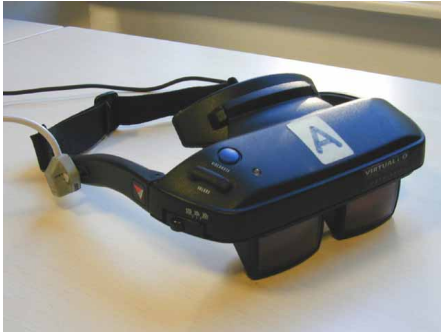
Figure 47. Virtual I/O i-glasses! head-mounted display with a mounted Polhemus Fastrak receiver.
