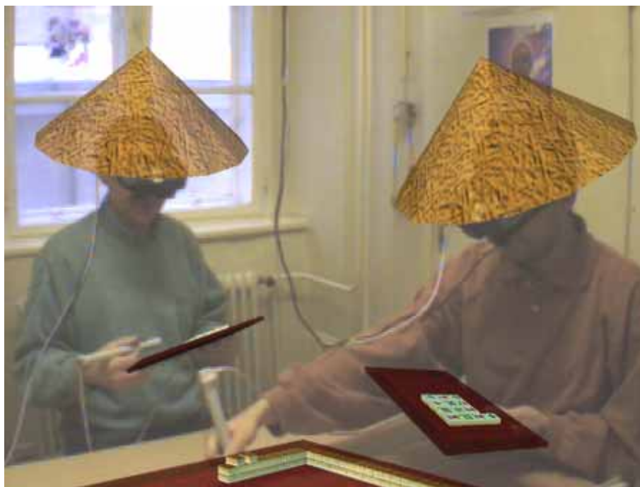
Figure 76. Mah-Jongg . The augmentation as seen from a third participant through the HMD.
