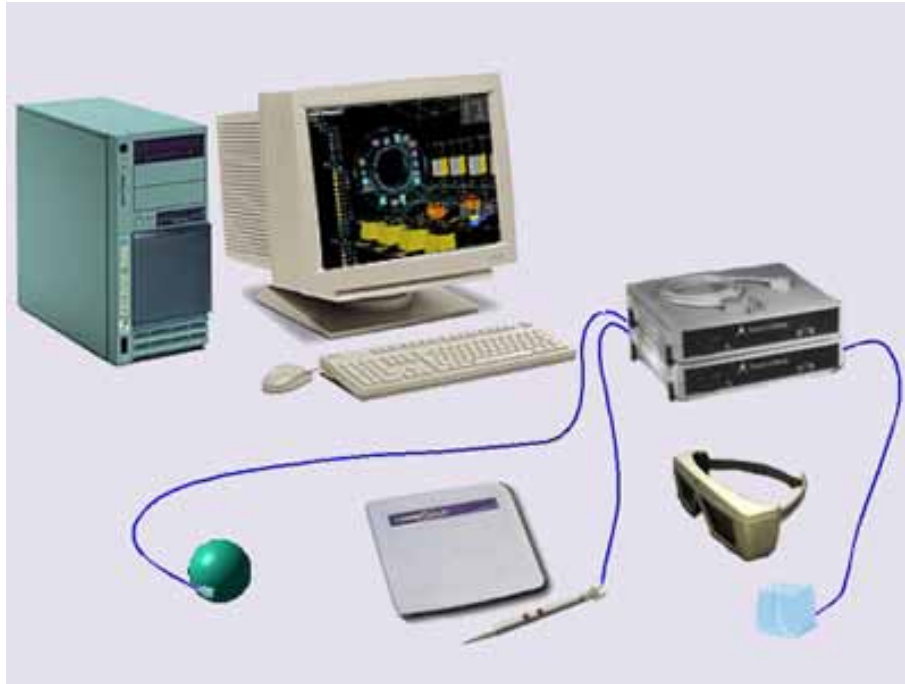
Figure 82. Personal Workspace – System setup showing components of the desktop environment. Navigation prop and the pen of the Wacom tablet are tracked using a MiniBird system.
