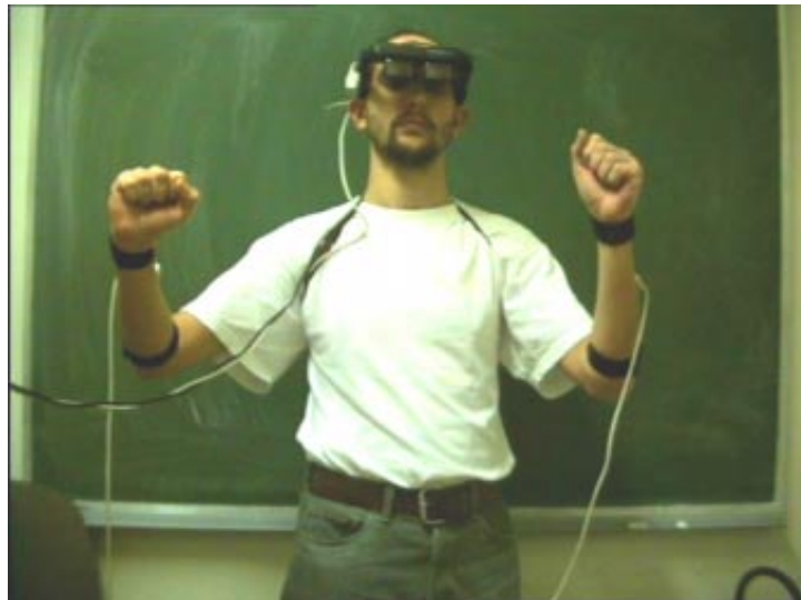
Figure 31: User with 4 sensors and HMD.
