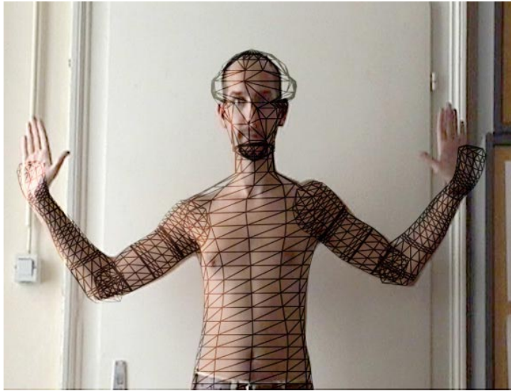
Figure 35: User with overlaid phantom avatar geometry.
