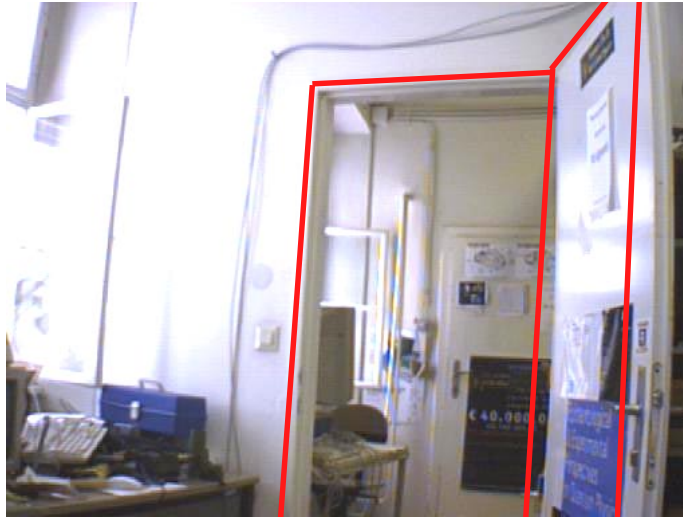
Figure 18: Lens distortion (red lines rendered with idealized camera)
