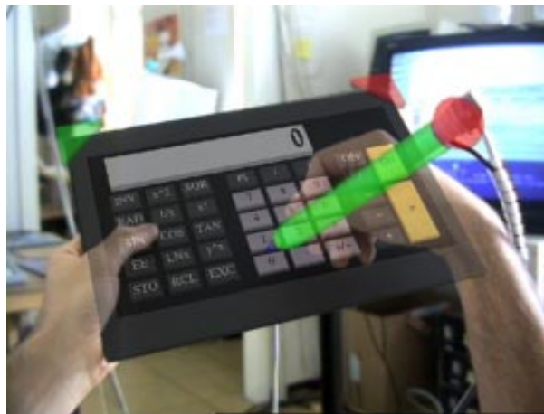
Figure 9: Calculator application overlaid onto PIP
