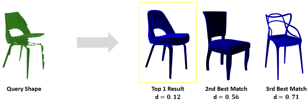
Figure 1: For instance level recognition on 3D data, the original instance of an object in a database is searched using a 3D scan of an object. A metric determines the distance d to all the shapes held in the database.
