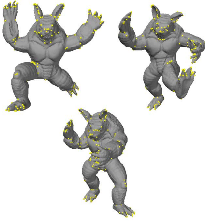
Figure 1: Examples of interest points detected with our method.
