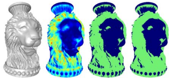
Figure 6: From left to right: The Lion Head model (39K vertices), roughness scalar field, clustering using K-Means (2 clusters), clustering using our MRF algorithm (2 clusters).
