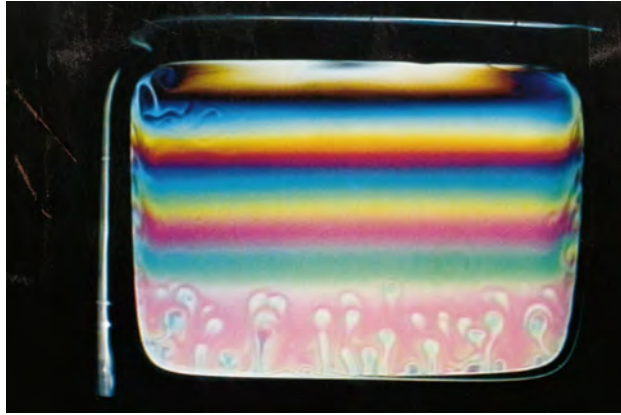
Figure 3.18: A vertical soap film with marginal regeneration. Picture taken from Nierstrasz and Frens’s work [86].
