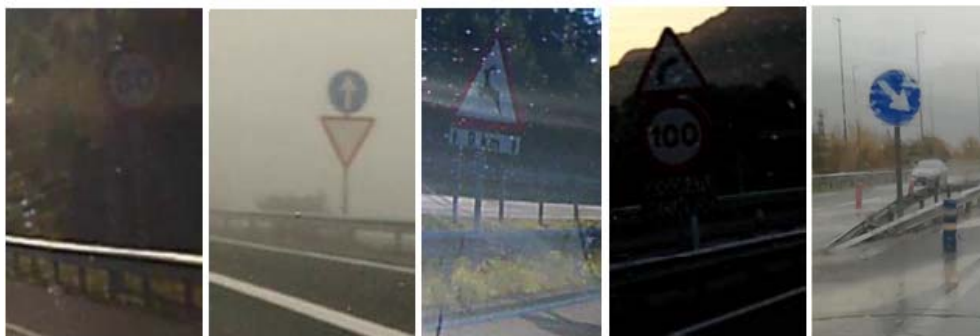
Figure 3-2. Ceit-TSR dataset. Sample images showing some of the challenging conditions: low contrast, fog, reflections, shadows, and heavy rain.
