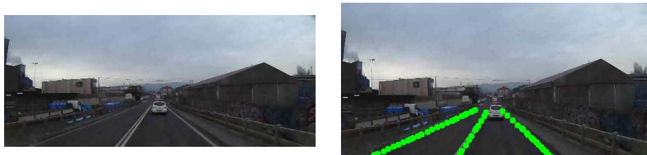
Figure 4-6. Machine learning-based lane condition assessment. Step 1, lane detection.
