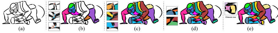
Figure 4.5: Method Overview. Given a vector line drawing (a), we first detect trivial stroke-wise intersections forming closed stroke loops (b, right). We then identify likely end-to-end (red) and T- (blue) junctions (b, left zoom-ins). With these pairs and their predictions, we construct primary junctions, supporting arbitrary valence (c, see left zoom-ins for examples). We proceed to identify secondary T-junctions formed by the remaining dangling endpoints and composite strokes (d, see left zoom-ins for example connections). In the final closure integrated step, we close remaining undesirable gaps by jointly evaluating classifier predictions and gap ratios along the boundaries of potential cycles (e, see the zoom-in for a connection classified as marginally negative in our primary step and accepted in this step). Input image ©The “Hero” artist Team under CC BY 4.0.
