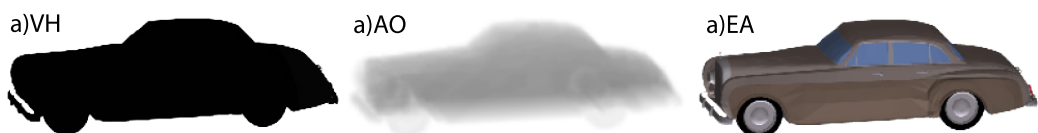
Figure 3.4: Different image formation models visual hull (VH), absorption-only (AO) and emission-absorption (EA).
