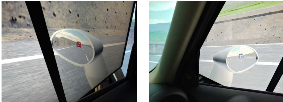
Figure 7.4: The driving simulator is in the process of being equipped with virtual side mirrors. They are implemented using rendered textures embedded into side mirror geometry on the side displays.
