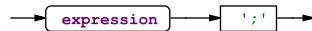
Figure A.5: The expression statement executes an expression. If the expression is missing, the statement becomes an empty statement.
