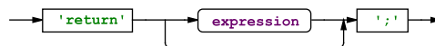
Figure A.14: The value of the expression is returned to the calling function. If the expression is omitted, the return value of the function is undefined.
