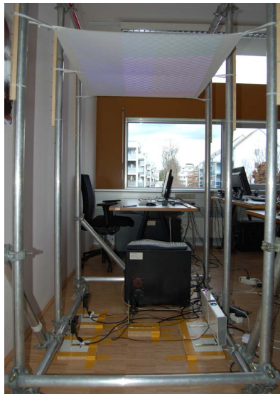
Figure 6.8: The test setup consists of a suspended sheet held in place by six rubber tapes that can be adjusted manually (top part). Vertical displacement of the scaled-down setup corresponds to two meters of the exhibition setup (see Figure 6.1). The four projectors and the wide-angle camera are located below the sheet (bottom part)
