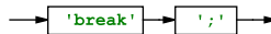
Figure A.13: The break statement belongs to the class of jump statements.
