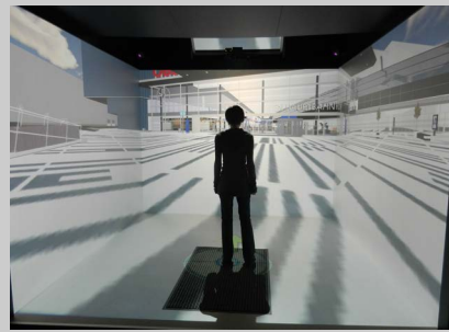
Figure 1.2: The DAVE in Graz resembles the shape of a box with 3.30m wide walls and consists of four projection walls (left, right, front, bottom) and four active stereo projectors being driven by eight computers.
