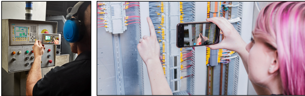
Figure 18 – On-site technicians receiving hand gestures from a remote collaborator through XMReality. Source: (XMReality, 2020)
