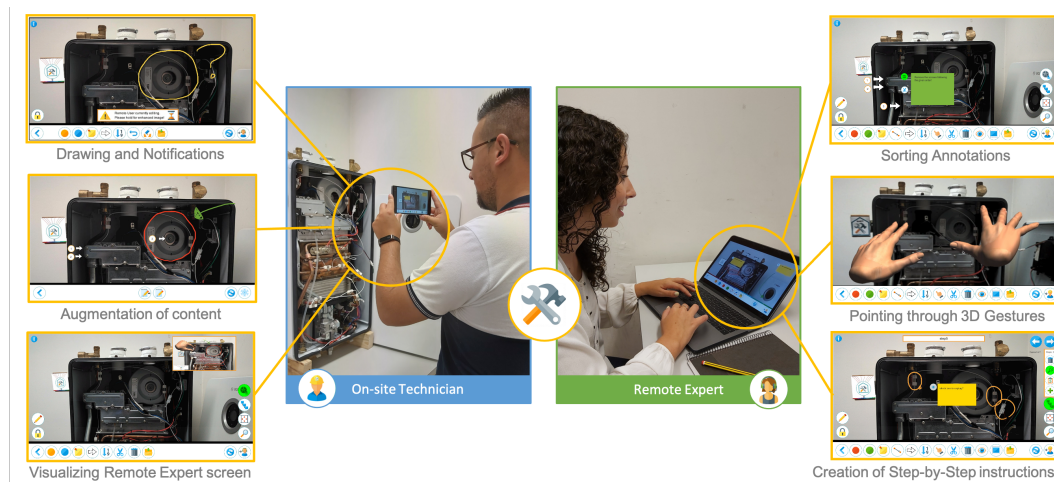
Figure 29 – Example of the prototype functions associated to the on-site technician (left: drawing and notifications; augmentation of content; visualizing remote expert screen) and the remote expert (right: sorting annotations; pointing through 3D gestures; creation of step by step instructions). Adapted from: (Marques et al., 2021).
