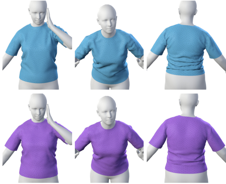
Figure 4.13: Comparison between a ground-truth physics-based simulation (top) and our data-driven method (bottom), on a test sequence not used for training (01_01 from [CMU]). Even though our method runs three orders of magnitude faster, it succeeds to predict the overall fit and mid-scale wrinkles of the garment.
