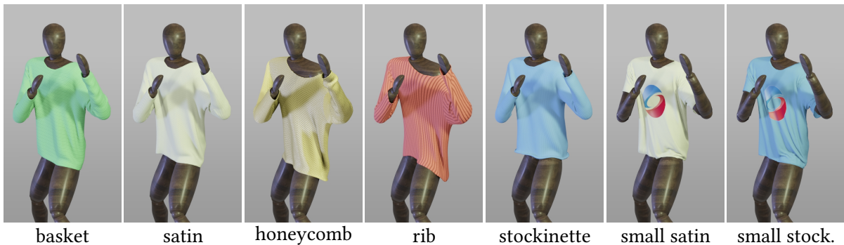
Figure 4.10: We demonstrate the effectiveness and the rich behavior of our homogenized models for all of our patterns on simulations of sweaters and t-shirts. This freeze frame highlights: stronger stretching resistance of woven fabric (basket and satin), the anisotropy of the rib, curling of the stockinette, and the folds of the small-scale patterns.
