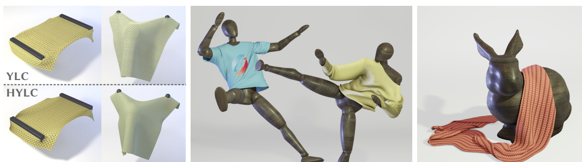
Figure 4.1: Left: A comparison between direct yarn-level simulation (YLC) and simulation with our homogenized model (HYLC); our homogenized model accurately captures the non-trivial elastic stretching and bending response of the fabric. Middle and right: Results simulated with homogenized continuum models of woven and knitted patterns; our method allows us to efficiently compute large-scale simulations where direct yarn-level simulation would be prohibitively slow.
