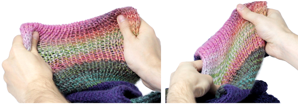
Figure 1.1: Photo of a stockinette knit being pulled in different directions. The individual loops of the knit interact in such a way that the fabric as a whole is compliant along the weft direction (here: horizontal) and more stiff along other directions.
