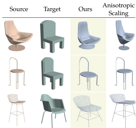
Figure 5.5.: Comparison of our method with anisotropic scaling. Our method better matches corresponding semantic parts.
