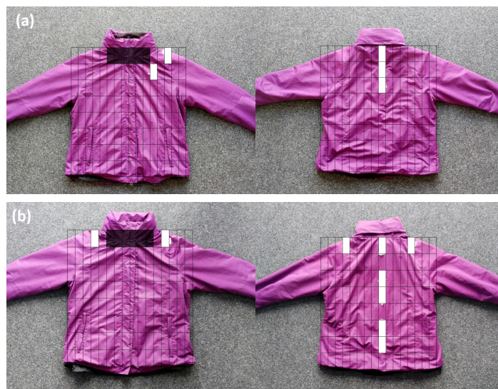
Figure 4.14.: Final prototype designs by two knowledgeable system designers. Tags mark sensor placement on front and back of jacket.
