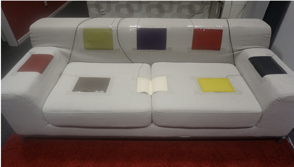
Figure 3.20.: Couch endowed with eight textile electrodes.
