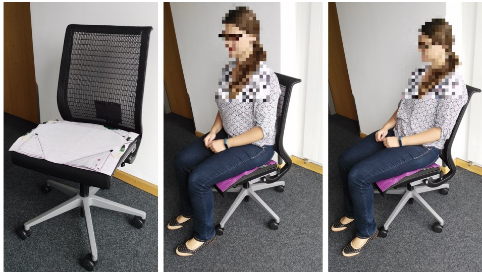
Figure 3.19.: Seat cushion prototype with person sitting upright and leaning back
