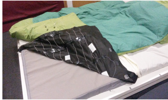
Figure 3.8.: Prototype bed sheet with wired grid
