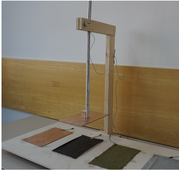
Figure 5.2.: Setup with measurement copper electrode adjusted at different distances in relation to various electrode materials
