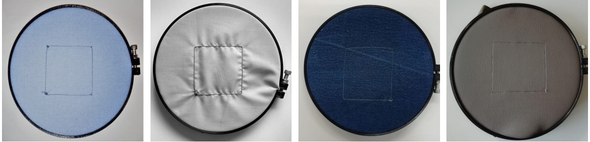
Figure 5.26.: Conductive thread stitched to different support materials: 100% cotton, 65% polyester and cotton 35%, stretch jeans (84% cotton, 14% polyester, 2% elastane), synthetic leather (100% polyurethane)
