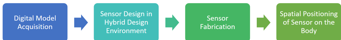
Figure 2.4.: Fabrication pipeline for on-body sensors by Steimle et al. [NS16].
