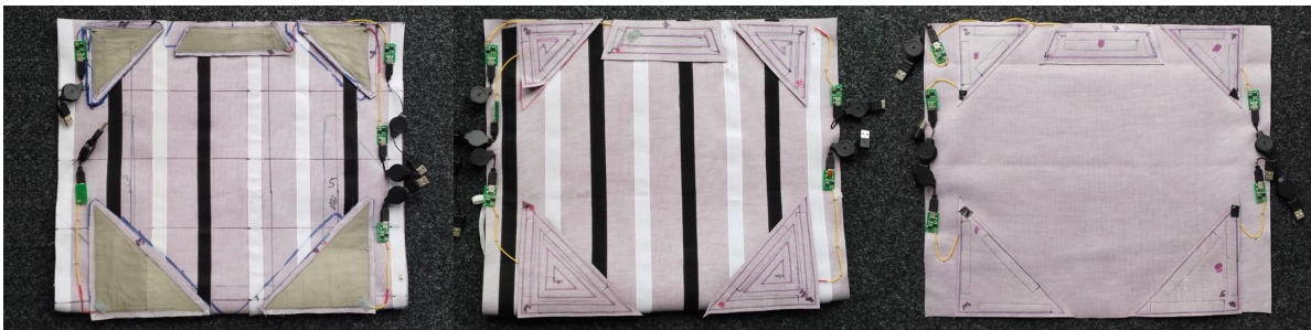
Figure 5.34.: Seat cushion prototypes with three electrode types: conductive fabric, conductive thread, and spiral
