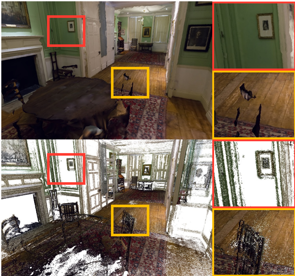
Figure 5.3: Top: Globally consistent reconstruction with RealityCapture [152]. Bottom: Same scene and viewpoint using COLMAP [160, 161]. We can clearly see that the featureless wall is completely missing from the COLMAP depth maps, but a smooth estimate is provided by RealityCapture. Conversely, the details of the back of the chair are only present in the COLMAP depth maps.
