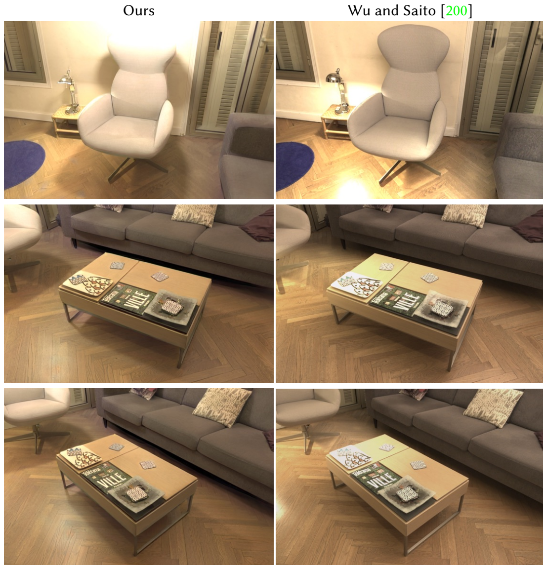
Figure 6.15: Single-image relighting comparison. We provide an indicative comparison with the single image method Wu and Saito [200] that has much less information than our multi-view input. We see that this method cannot reproduce shadows of complex objects such as the armchair, nor the view-dependent glossy effects on the hardwood floor.
