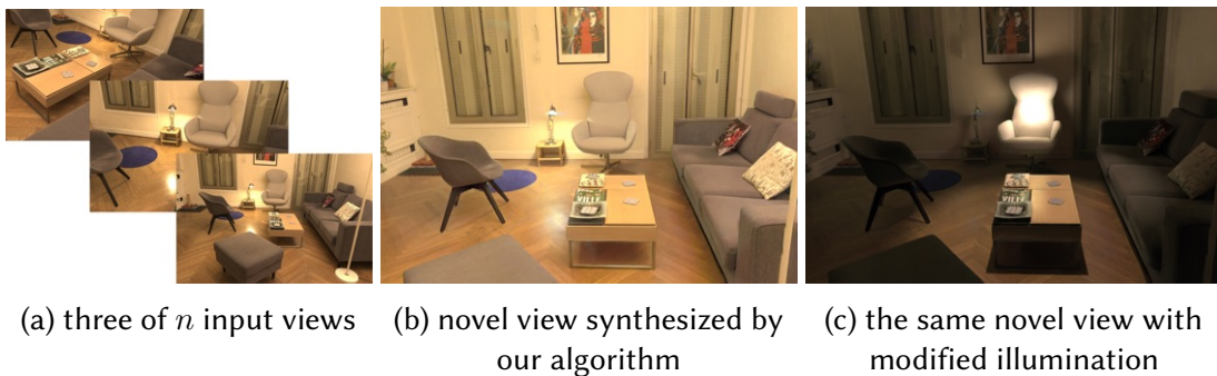
Figure 6.1: Our neural algorithm takes as input a multi-view capture of a real scene under a single lighting condition (a). It re-renders the scene from novel viewpoints, accounting for view-dependent glossy effects, e.g., on the floor (b) and on the table (c), allowing free-viewpoint navigation. Our network internally builds an implicit representation of the scene materials, based on complex input feature maps we compute with a novel hybrid image- and physically-based rendering algorithm. This enables a user to insert new lights in the scene and/or turn off the original illumination; the network produces a new rendering of the scene under the modified lighting (c). Note how the light – that was on in the input photos – has been turned off with our method.
