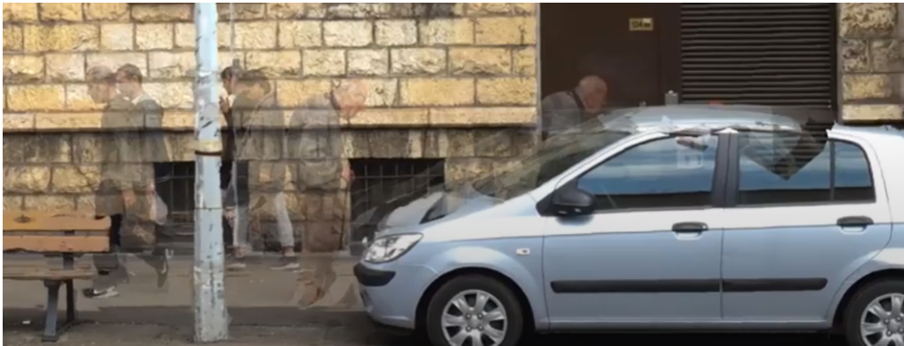
Figure 1.5: Unstructured Lumigraph rendering[19] of a scene captured with moving people and specular objects. When sampling the input images, moving people are blended with the background leading to ghosting artifacts. The specular parts of the car are badly reconstructed leading to severe visual artifacts.
