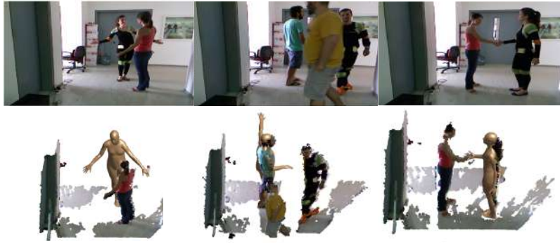
Fig. 3.7: Experiments from [286] dataset show different occlusions caused by external agents. Multi-person does not introduce confusion. In the middle, the arm has been placed to a different solution for the occluded part, but consistent with acquired view.
