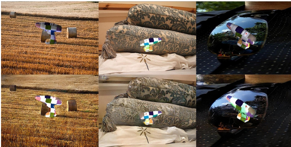
Figure 4.21: Checkerboard surface reconstruction results as required by surface rendering method 4). Top row: target image. The input to the network is a Laplace filtered version (confer Figure 4.14c) Bottom row: output of the PIX2PIXHD model trained to reconstruct the checkerboard pattern and applied to the whole image.
