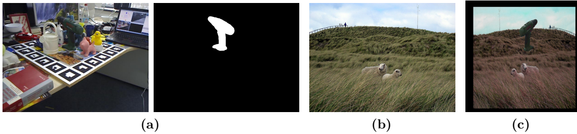
Figure 2.7: A standard data augmentation pipeline: given (a) an image with segmentation mask and (b) a random background, (c) a new training sample is generated by composition while also varying hue and scaling
