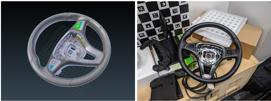
(b) CNN training with CAD geometry: Given the CAD geometry of an object ( left ) detect the object and its pose in real images ( right )
