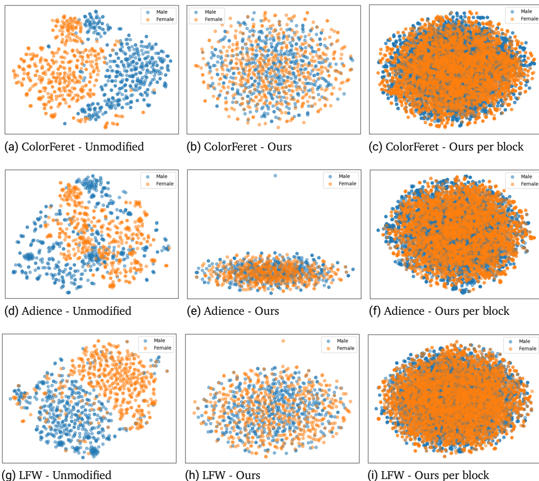
Figure 5.38.: Visualization of different face representations of the three databases, ColorFeret (5.38a - 5.38c), Adience (5.38d-5.38f), and LFW (5.38g-5.38i). For the visualizations, 500 female and 500 male identities were chosen randomly and their templates are reduced to two dimensions using t-distributed stochastic neighbour embedding (t-SNE) [MH08]. The first row (a, d, g) shows the t-SNE plots for the original facenet embeddings. The second row (b, e, h) shows the same plots for templates modified by our PE-MIU approach. The last row represents the t-SNE plots created from each block of the templates. The lower separability introduced by PE-MIU in comparison to the unmodified templates is demonstrated by the increasingly overlapping samples.
