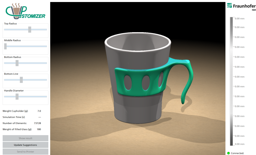
Figure 6.4.: Interactive exploration of a given design space using a CC-solid model with five parameters, linked with a finite element simulation based on tetrahedra.
