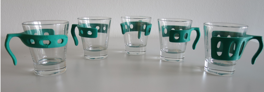
Figure 6.7.: Print-outs of five different cup holders, customized and simulated with the application presented here. All five passed the validation.
