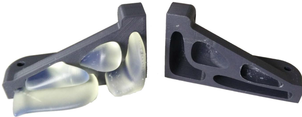
Figure 6.13.: Demo print-out of the bracket including four interactively designed subdivision-based cavities.
