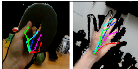
Figure 5.13: Failures in the hand localization step (left) or fast motion that leads to misalignment in the colored depth image (right) can cause incorrect pose estimates.
