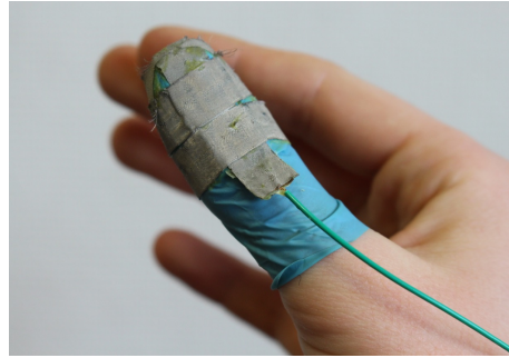
Figure 8.7: Automatic ground-truth annotation of thumb-to-finger touch using a capacitive finger glove, built out of nitrile rubber with conductive fabric affixed around the tip of the finger.
