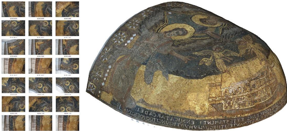
Figure 46. Point cloud from a set of 2D poses reconstructed via dense-image matching using the software ContextCapture v 4.4.6, Bentley Systems, Exton, United States [17].
