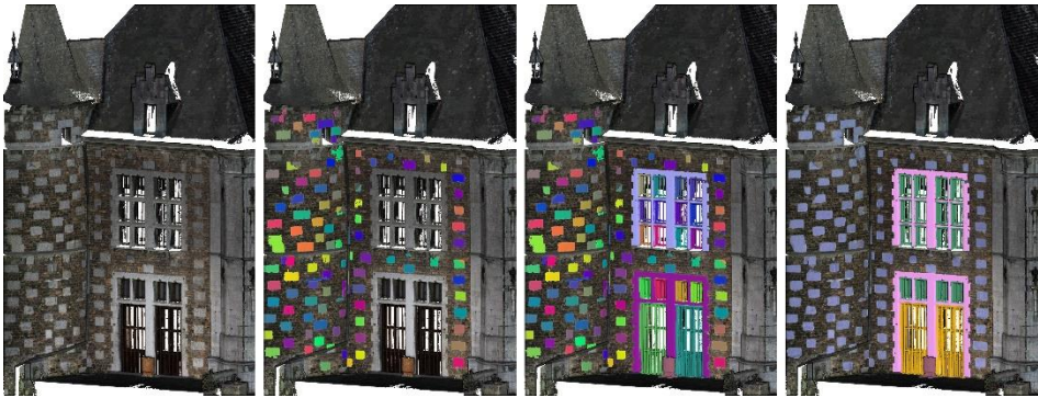
Figure 54. Ontology-based classification of the South-South-West façade of the castle of Jehay. From left to right: the façade studied; the result of the segmentation (stones only); the result of the full segmentation; the result of the classification for quasi-planar objects of interest.
