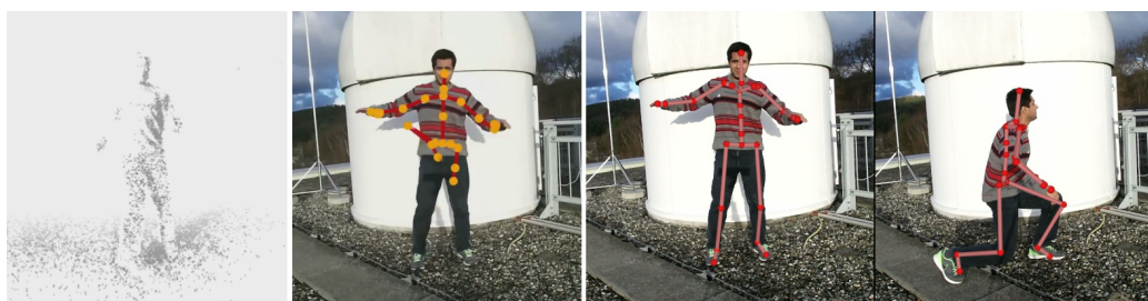
Figure 8.6: VNect, being based on RGB camera input succeeds in strong illumination and sunlight (center right and right), while the IR-based depth estimates of the Microsoft Kinect are erroneous (left) and depth-based tracking fails (center left).
