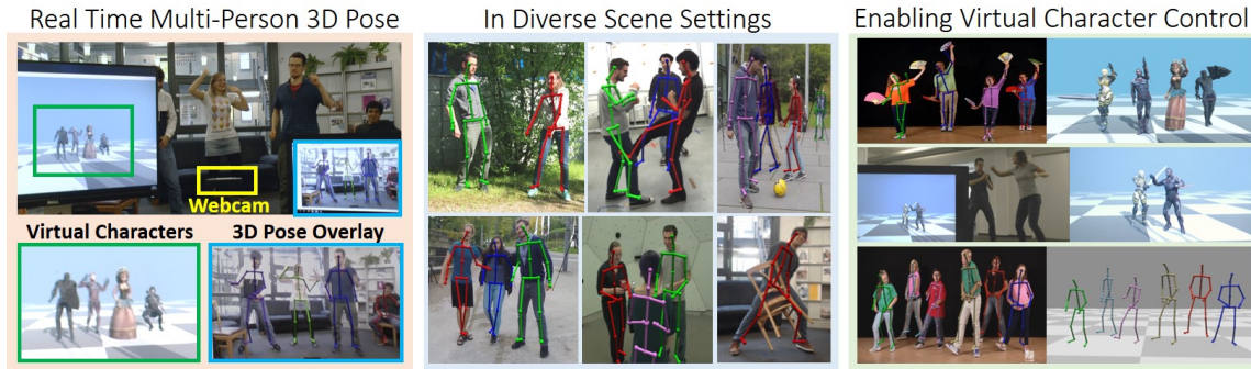
Figure 8.9: XNect, the real-time monocular RGB based 3D motion capture system provides temporally coherent estimates of the full 3D pose of multiple people in the scene, handling occlusions and interactions in general scene settings, and localizing subjects relative to the camera. The design allows the system to handle large groups of people in the scene with the run-time only minimally affected by the number of people in the scene. The method yields full skeletal pose in terms of joint angles, which can readily be employed for interactive character animation.
