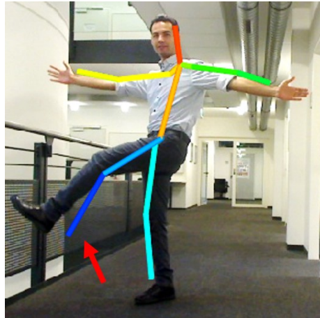
Figure 5.1: The 3D predictions resulting from direct image to 3D pose vector regression do not match the extent of articulation of the input image, and tend towards the average pose of the training corpus.
