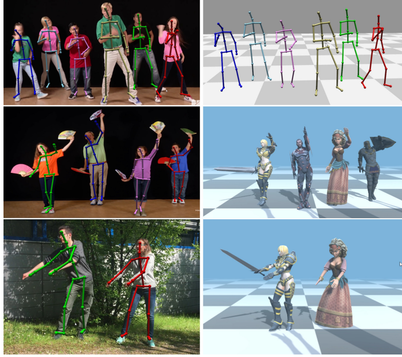
Figure 8.10: Virtual Character Control: The temporally smooth joint angle predictions from XNect Stage III can be readily employed for driving virtual characters.
