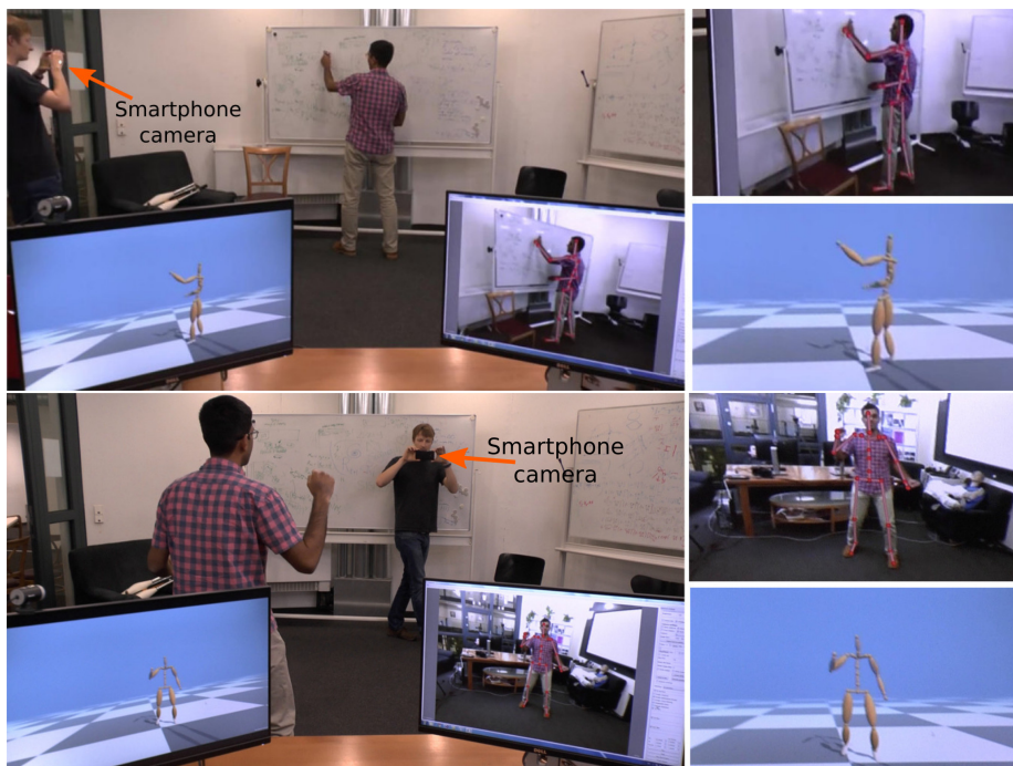
Figure 8.8: Handheld recording with a readily available smartphone camera (left) and the estimated pose from VNect (right), streamed to and processed by a GPU enabled PC.
