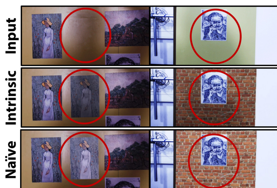
Figure 3.15: Realistic texture replacement: a virtual painting (left) is added, and a brick texture (right) applied. The textures realistically interact with the illumination (red circles). With a naïve texturing approach, shadows are lost.
