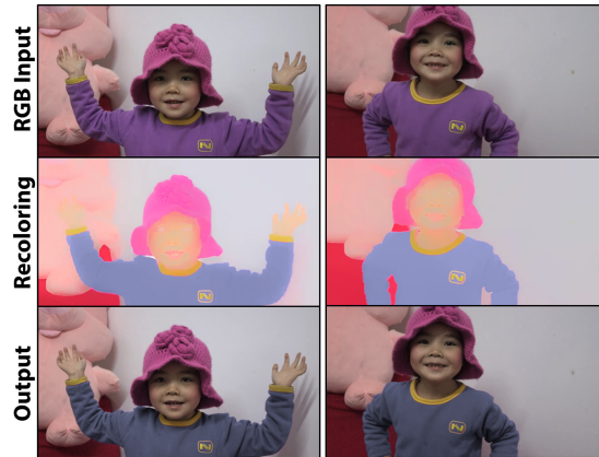
Figure 3.13: Reflectance recolouring on the GIRL sequence. The girl’s is recoloured in real-time using this intrinsic decomposition approach. Note that the shading detail is preserved.
