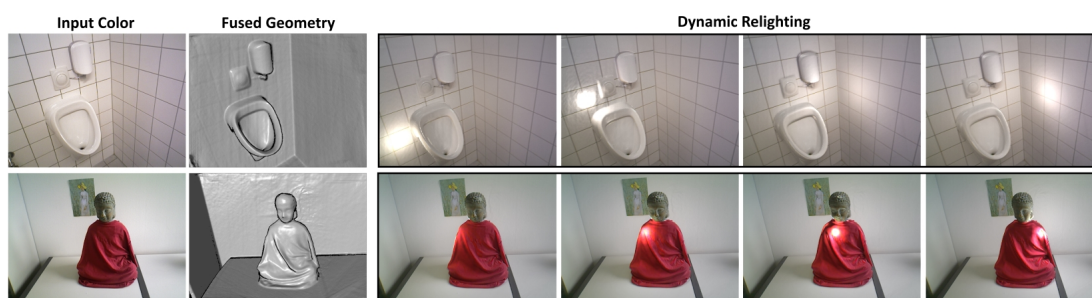
Figure 4.10: Dynamic geometry-based relighting. A virtual shading image is generated by rendering the scene geometry under a new light source. The resulting shading map is blended with the shading layer before recombining it with the reflectance to obtain a relighting effect.
