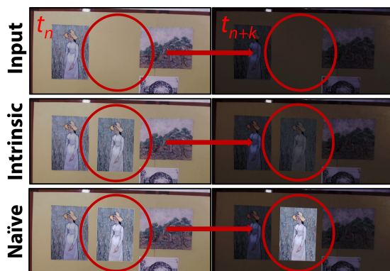
Figure 3.16: Realistic texture replacement: a virtual painting is added to the wall. The textures realistically reflect the illumination change (red circles) caused by dimming the lights. Note that a naïve texturing approach leads to unrealistic results.
