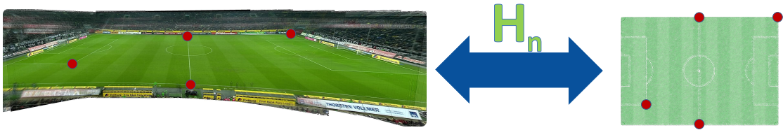
Figure 3.3.7: The chosen points for the transformation of the panoramic (left) into the normalized (right) view must allow referencing distances in both directions of the main axes. Afterwards, a calculated homography H_n enables the transformation of panoramic view into normalized view and vice versa.
