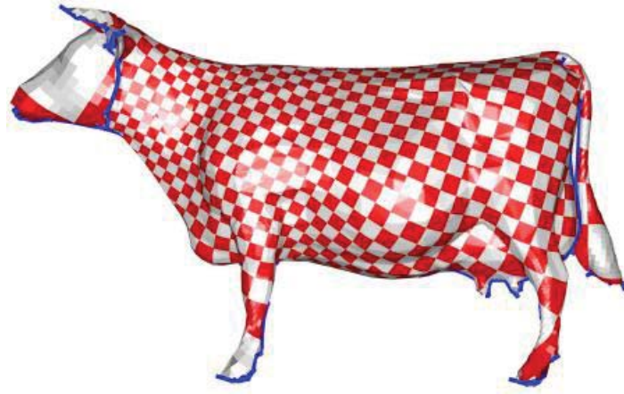
Figure IV-C.1.9: Texture map for the Cow dataset ( \alpha = 0 ). Area distortion is more noticeable in the head, legs and tail.
