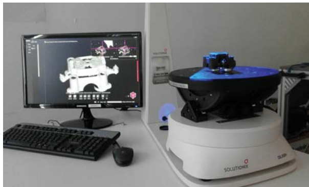
Figure IV-C.4.8: Acquisition of 3D point cloud data through an optical 3D scanner
