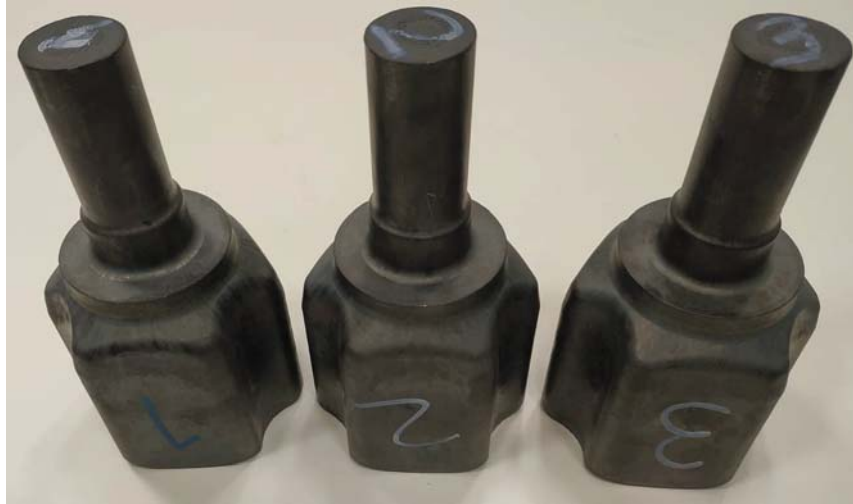
Figure IV-E.2.11: Cold workpieces used to run the ANOVA R&R test. The three workpieces share the same CAD reference.
