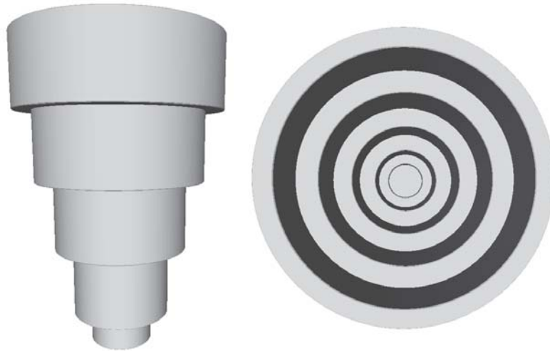
Figure IV-E.2.5: Front and top views of the calibration object geometry.
