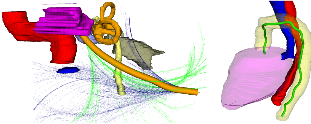
Figure 5.3.: Left: Bidirectional RRTs grow two search trees - one from the initial region (blue), the other from the goal region (green)- and attempts to connect them in between. A successful connection results in a feasible nonlinear trajectory. Right: Catheter insertion into the heart's coronary vessels with the help of guidewires enables easier access. Navigating through the aorta (yellow) is the first challenge during such interventions.
