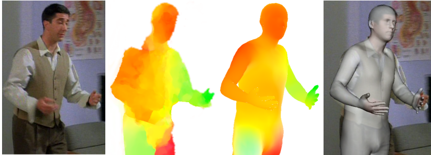
Figure A.1: Following our main idea we compute the optical flow between two consecutive frames and match it to an optical flow field estimated by our proposed optical flow renderer. From left to right: input frame, color-coded observed flow, estimated flow, resulting pose.
