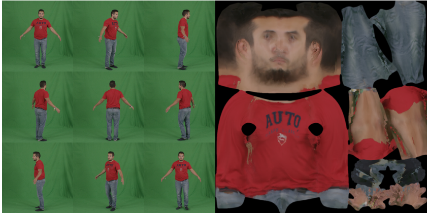
Figure B.4: We back-project the image color from several frames to all visible vertices to generate a full texture map.
